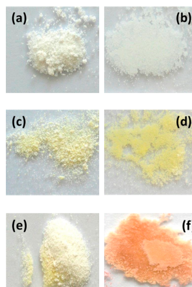
Figure 4. Photographs of HMB/PUF (a, b) and CA/PUF (c, d) microcapsules before (a, c) and after (b, d) breaking them by shearing between glass slides. Also shown is a mixture of HMB/PUF and CA/PUF microcapsules in their pristine (e) and broken (f) state.
